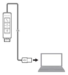
The USB Audio Processor is automatically powered on upon inserting into the USB port of the computer.
