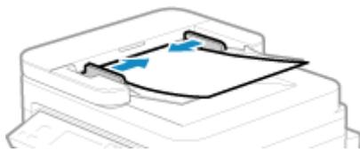
Slide guides that are aligned but too loose or too tight can cause misfeeds or a paper jam.
