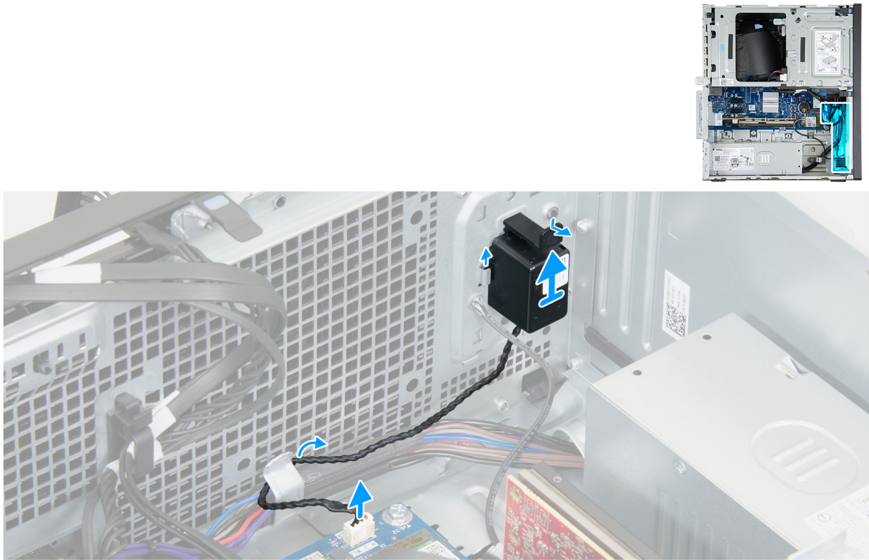
Figure 25. Removing the internal speaker
