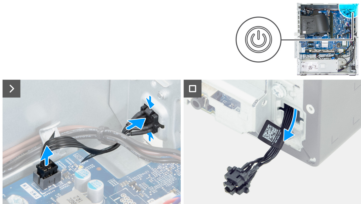
Figure 50. Removing the power button
