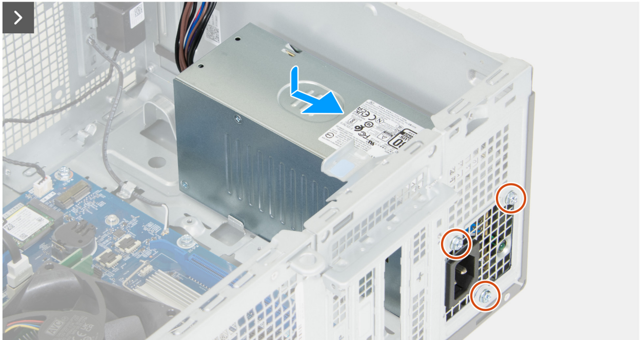
Figure 64. Installing the power-supply unit
