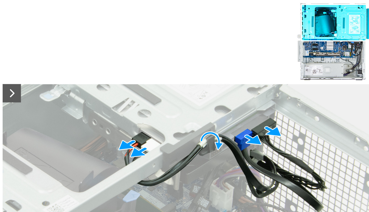
Figure 42. Removing the drive bay
