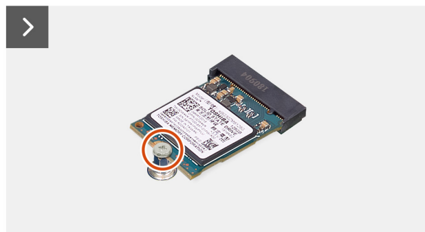
Figure 29. Removing the M.2 2230 solid-state drive
