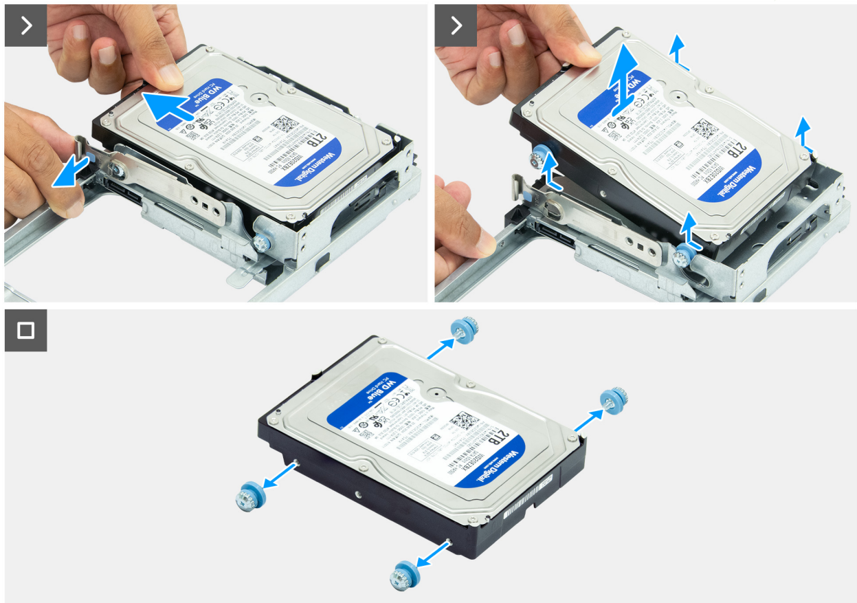
Figure 46. Removing the hard drive
