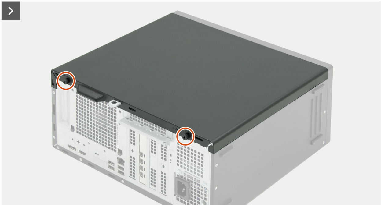
Figure 13. Removing the left-side cover
