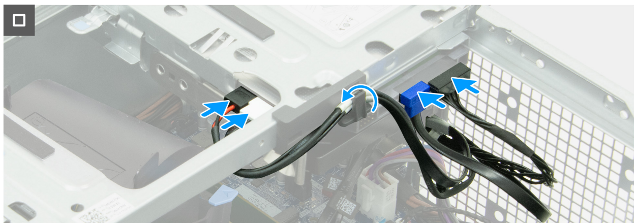
Figure 45. Installing the drive bay
