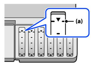
7. Align the top of the ink bottle with the filling port, and then insert it straight into the port to fill ink until it stops automatically at the upper line.
