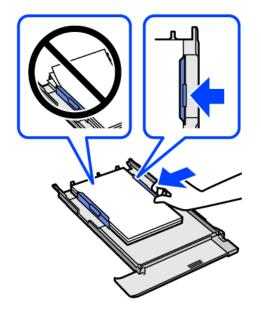
12. Align the edges of the paper and slide the edge guides to the edges of the paper.
