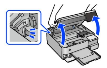
4. Check if the translucent film is smeared. Smears are easier to see if you use a light.If there are smears (such as finger marks or grease) on the translucent film (A), go to the next step.
