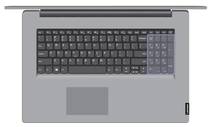
Some Lenovo computers includes a dedicated numeric keypad on the far right of the keyboard. The keypad is used for entering numbers and operators quickly.
