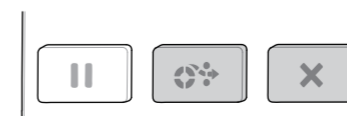
4. Verify that your printer is able to print a configuration label by holding both FEED and CANCEL for 2 seconds.
