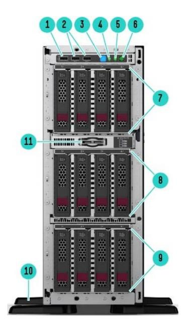
Front View - LFF chassis with optional Gen10 4LFF HDD Cage Kits shown (Tower mode)
