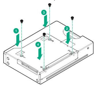
**3.** Remove three drive screws from the front panel.
