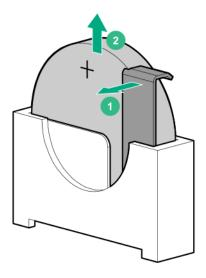
3. Slightly push the metal lab, and then install the new system battery in the socket.
