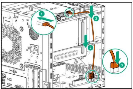
**5.** Bundle the extra length of the SSD power and SATA cables, and then secure them in the cable ties.
