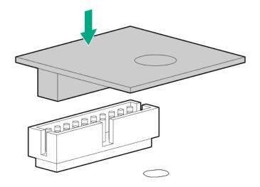
**3.** Install the TPM security rivet by pressing the rivet firmly into the system board.
