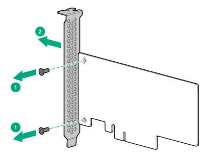
2. Install the low-profile bracket on the expansion board.
