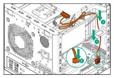
**f.** Bundle the extra length of the SATA Y-cable and the power supply P3 cable, and then secure them in the cable tie.
