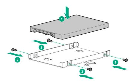
2. Install the SSD assembly in the media bay, and then secure it with the screw.
