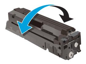
Install the new toner cartridge. Make sure that the color chip on the cartridge matches the color chip on the drawer.
