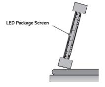
3 Place the product with the LED package screen facing down. To protect the screen, lay the protective pad in the box on the floor.
