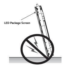
2 If the product is tilted towards the edge of the LED package screen after the brackets on the corners are removed, the bottom (corner) of the product may be damaged.
