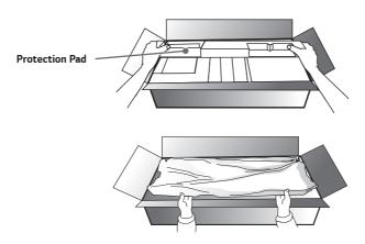
2 To stand the product upright, hold it on both sides so that the LED package screen does not touch the floor.
