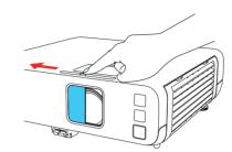
4 Press the opening power button on the projector or remote control. The projector beeps, and the Status light flashes blue and then stays on.
