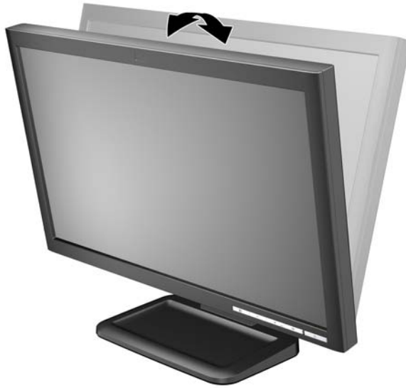
Figure 3-7 Tilting the Monitor
