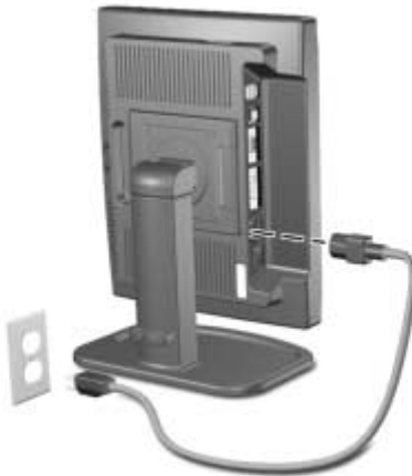
Connecting the Power Cable
