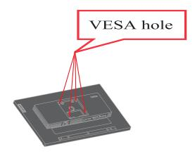
Step 5: Attach the LCD display to the wall, following the instructions in the wallmounting kit. For use only with UL/GS Listed Wall Mount Bracket with minimum weight/load:10.44 kg
