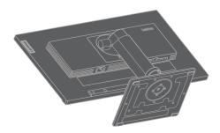
Step 4: Attach the mounting bracket from the VESA compatible wall mounting kit (100mm  $\,$ x100mm distance), VESA Mounting Screw M4  $\,$ x 10 mm.
