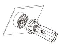
® Bracket Adjustment-Loosen the fixed ring to adjust the view angle of the camera. After you get the optimum angle of view, tighten the fixed ring to complete the installation.
