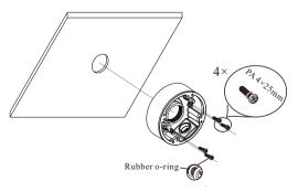
4 Mount the rubber plug to the gap of the mounting base and fasten the camera onto the mounting base.
