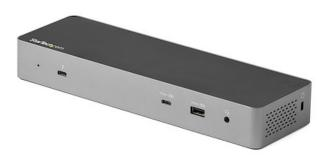
A high-performance Thunderbolt 3 Certified docking station with USB Type-C compatibility featuring dual monitor 4K 60Hz DSC support from either Dual or dual HDMI 2.0 video outputs, 96W Power Delivery (compatible with 100W laptops), 5x USB 3.2 Hub with 2x BC 1.2 fast charging ports, gigabit Ethernet & headset ports.
