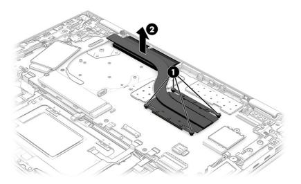
**3.** Thoroughly clean the thermal material from the surfaces of the heat sink and the system board components each time the heat sink is removed. Replacement thermal material is included with the heat sink and system board spare part kits. The following illustration shows the replacement thermal material locations.
