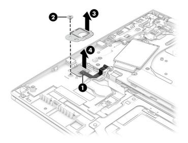
Reverse this procedure to install the fingerprint reader board.
