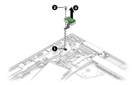
Reverse this procedure to install the audio jack module.
