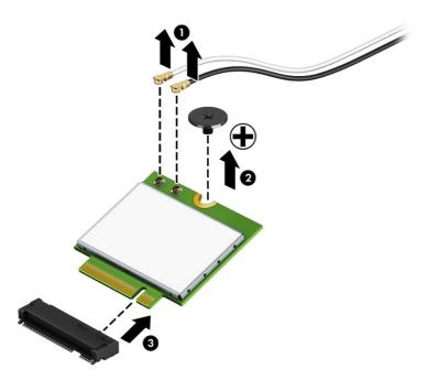
**3.** If the WLAN antenna is not connected to the terminal on the WLAN module, install a protective sleeve on the antenna connector, as shown in the following illustration.
