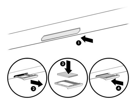
To remove the SIM card, press in gently on the SIM card access tray to disengage the SIM lock, and the tray will pop out of the slot. Remove the SIM card. Replace the tray in the computer and press in gently on the tray until it is firmly seated.
