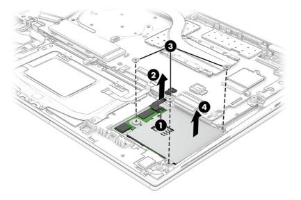
Reverse this procedure to install the card reader board.
