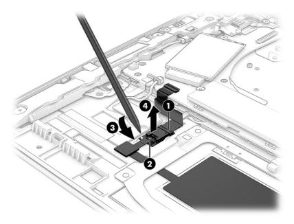
Reverse this procedure to install the NFC module.
