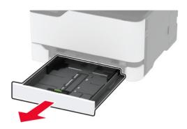
2 Remove the used manual feeder.
