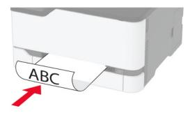
• Load envelope with the flap side down and against the right side of the paper guide.
