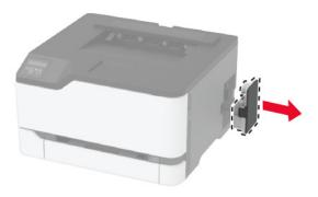
**Note:** To avoid spilling the toner, place the bottle in an upright position.
