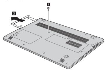
6 Remove the screw 3, then remove the optical drive bracket in the direction shown by arrow 4.
