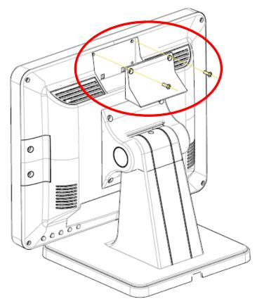
3. Mount the second display set to the touch monitor and install screws to secure. Plug USB cable into monitor USB port.
