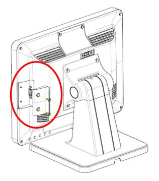
2. Insert the MSR module into the MSR USB port on the monitor.
