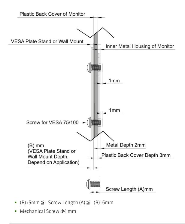
**Caution:** Please follow the Screw Specification in diagram for assembling VESA plate stand or Wall mounts plate into monitor back cover. Otherwise, it may cause mechanical damage.
