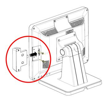
3. Make sure the MSR module is properly inserted and then install the 2 screws to secure it.
