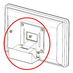
2. Remove the display mount cover from the monitor.
