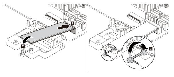
Figure 37. Installing the M.2 solid-state drive
