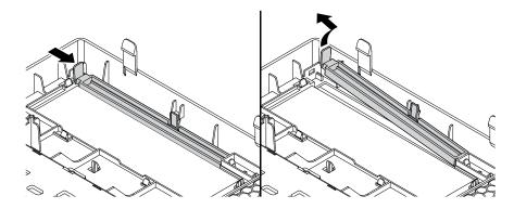
Figure 17. Removing the plastic shield
