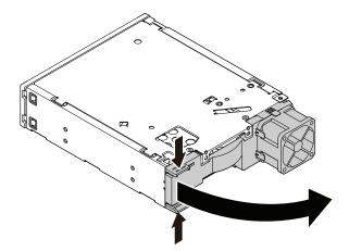
Figure 67. Opening the enclosure from the rear
