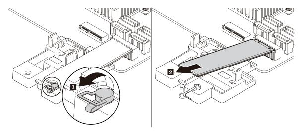
Figure 34. Opening the retention latch and removing the M.2 solid-state drive
