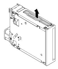
Figure 50. Removing the retainer
