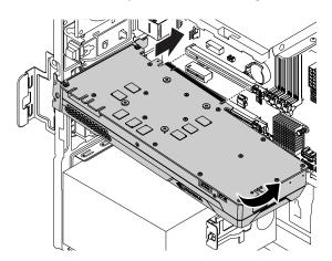
Figure 31. Installing a new full-length PCIe card
