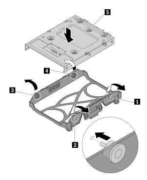
Figure 92. Installing the 2.5-inch storage drive with the storage-drive converter into the bracket
