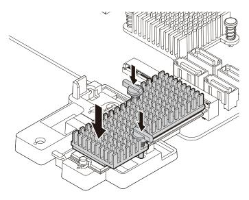
Figure 38. Installing the heat sink onto the plastic holder
