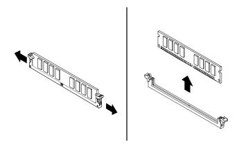
Figure 46. Removing a memory module
