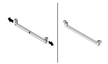
Figure 47. Opening the retaining clips
