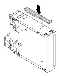
Figure 51. Installing the retainer
