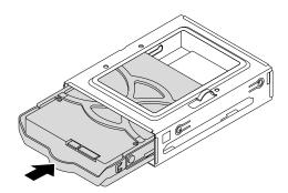
Figure 97. Installing the storage drive
