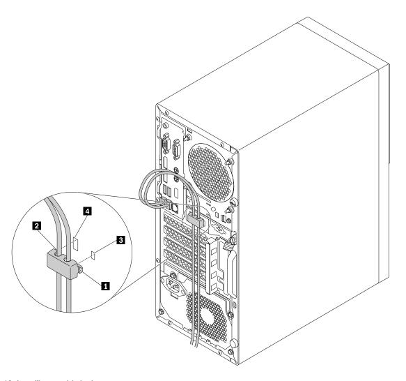
Figure 10. Installing a cable lock
