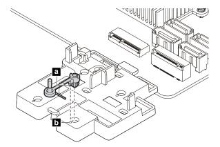
Figure 36. Installing the retention latch
