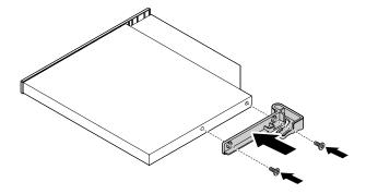
Figure 19. Installing the bracket
