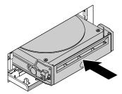
Figure 57. Installing the 3.5-inch storage drive into the front-access storage enclosure
