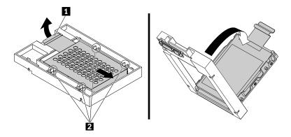
Figure 61. Removing the adapter from the converter
