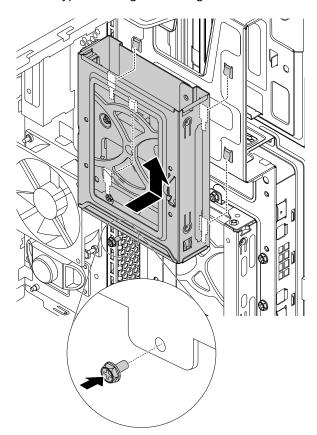
Figure 106. Installing the type-1 storage-drive cage
