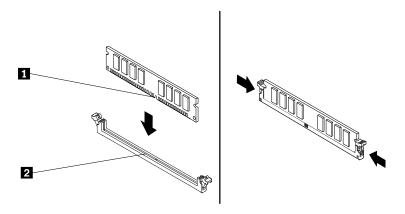
Figure 48. Installing a memory module
