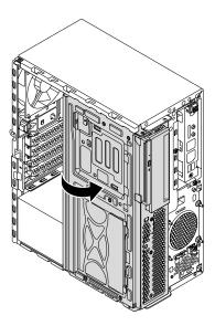
Figure 14. Pivoting the drive bay assembly outward
