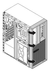
Figure 13. Removing the front bezel
