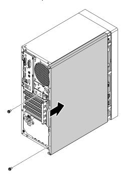
Figure 115. Reinstalling the computer cover
