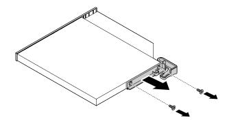
Figure 16. Removing the bracket
