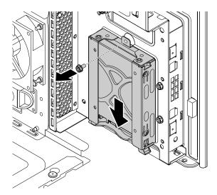
Figure 107. Removing the type-2 storage-drive cage
