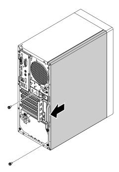
Figure 12. Removing the computer cover
