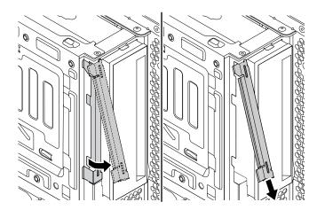
Figure 18. Removing the metal shield
