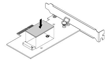
Figure 42. Installing the thermal pad
