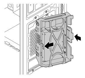
Figure 93. Installing the 2.5-inch storage drive
