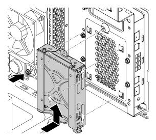
Figure 111. Installing the type-2 storage-drive cage
