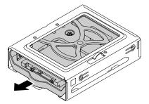
Figure 100. Removing the 2.5-inch storage drive
