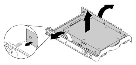
Figure 74. Removing the storage-drive converter from the 3.5-inch storage-drive bracket
