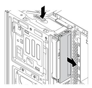
Figure 49. Removing the flex storage enclosure
