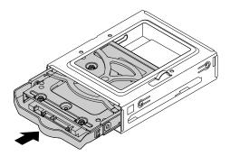
Figure 105. Installing the 2.5-inch storage drive into the type-1 storage-drive cage
