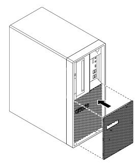
Figure 116. Reinstalling the dust shield
