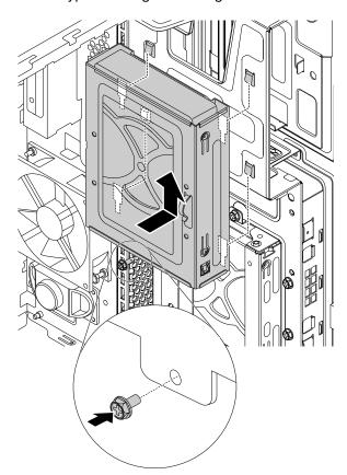
Figure 98. Installing the type-1 storage-drive cage
