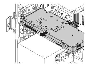
Figure 28. Removing a full-length PCIe card
