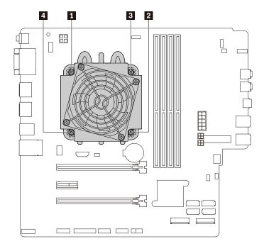
Figure 112. Removing the heat-sink-and-fan assembly
