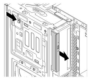
Figure 15. Removing the slim optical drive
