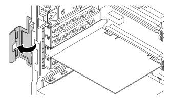
Figure 22. Rotating the PCIe card retainer
