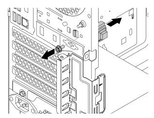
Figure 82. Removing the cover presence switch
