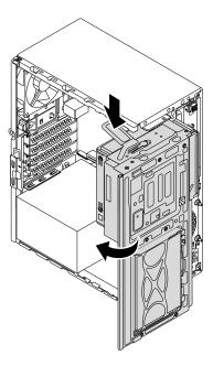
Figure 113. Pivoting the drive bay assembly downward
