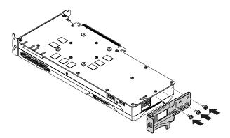
Figure 30. Installing a full-length PCle card bracket
