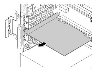
Figure 23. Removing a PCIe card
