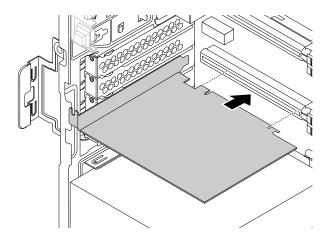
Figure 24. Installing a new PCIe card
