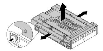
Figure 60. Removing the 2.5-inch storage drive from the bracket
