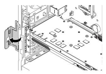
Figure 27. Rotating the PCIe card retainer
