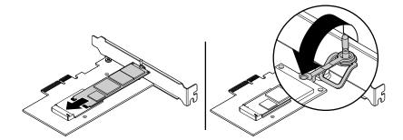
Figure 43. Installing the M.2 solid-state drive
