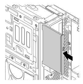
Figure 20. Installing the slim optical drive
