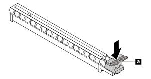
Figure 21. Disengaging the card retaining latch
