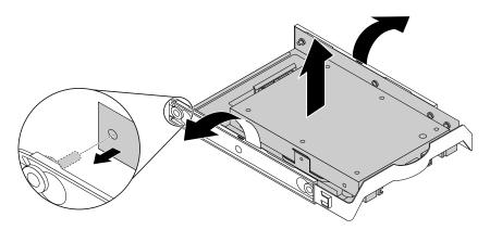
Figure 89. Removing the storage-drive converter from the 3.5-inch storage-drive bracket
