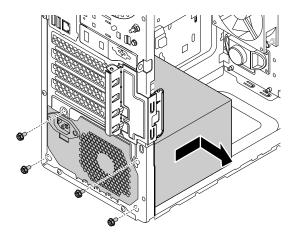
Figure 84. Removing the power supply assembly
