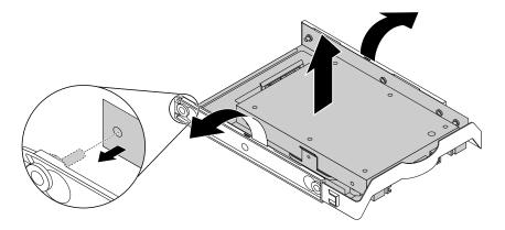
Figure 101. Removing the storage-drive converter from the storage-drive bracket
