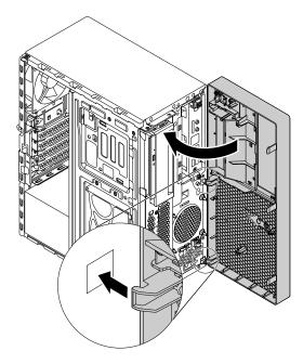
Figure 114. Reinstalling the front bezel
