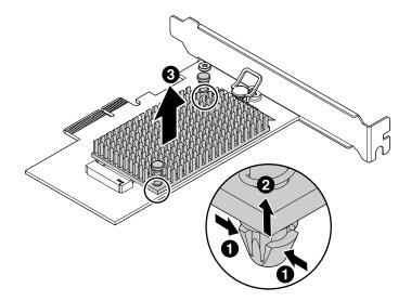
Figure 40. Removing the heat sink from the M.2 solid-state drive adapter
