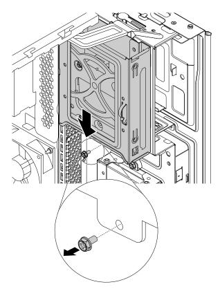
Figure 99. Removing the type-1 storage-drive cage
