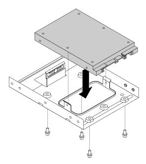
Figure 91. Installing the new 2.5-inch storage drive into the storage-drive converter
