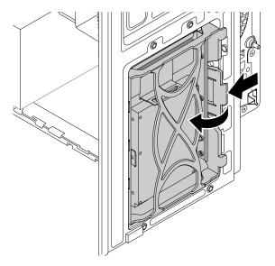
Figure 88. Removing the 2.5-inch storage drive with 3.5-inch storage-drive bracket
