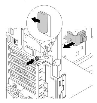
Figure 83. Installing the cover presence switch
