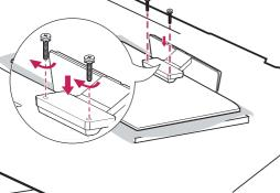
3 Use the screws to secure the stand to the back of the product as shown below.
