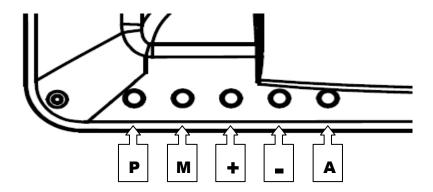
There are 5 keys for user to set up the monitor. The following describes functions of these Keys.
