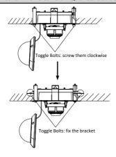
Figure 2-15 Fix the Bracket in Ceiling
