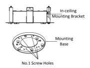
Figure 2-13 Install Mounting Base
