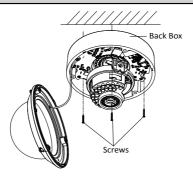
Figure 2-7 Secure the Camera
