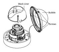
Figure 2-2 Remove the Bubble and Black Liner (Type II Camera)
