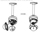
Figure 2-27 Secure Black Liner and Bubble
