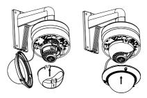
Figure 2-22 Secure Black Liner and Bubble
