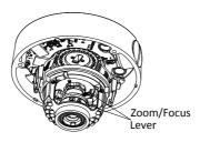
Figure 2-35 Zoom/Focus Lever (Type I Camera)
