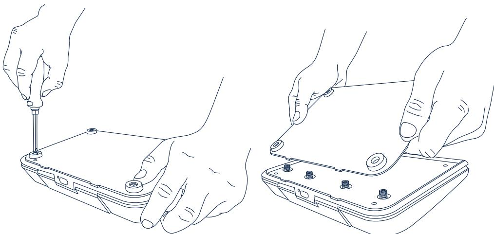
Loosen four screws with a Phillips head (PH) screwdriver.
