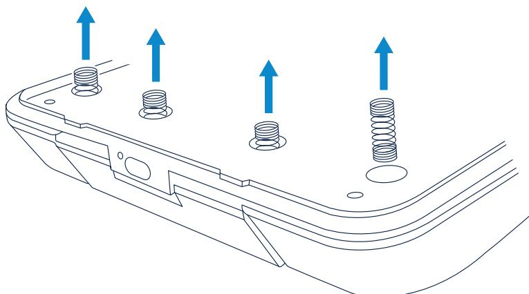
Adjust pedal pressure with the included spring tension sets.
