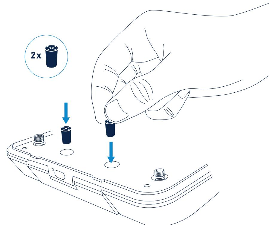
Lock the middle pedal with the included stoppers to convert it into a convenient footrest.
