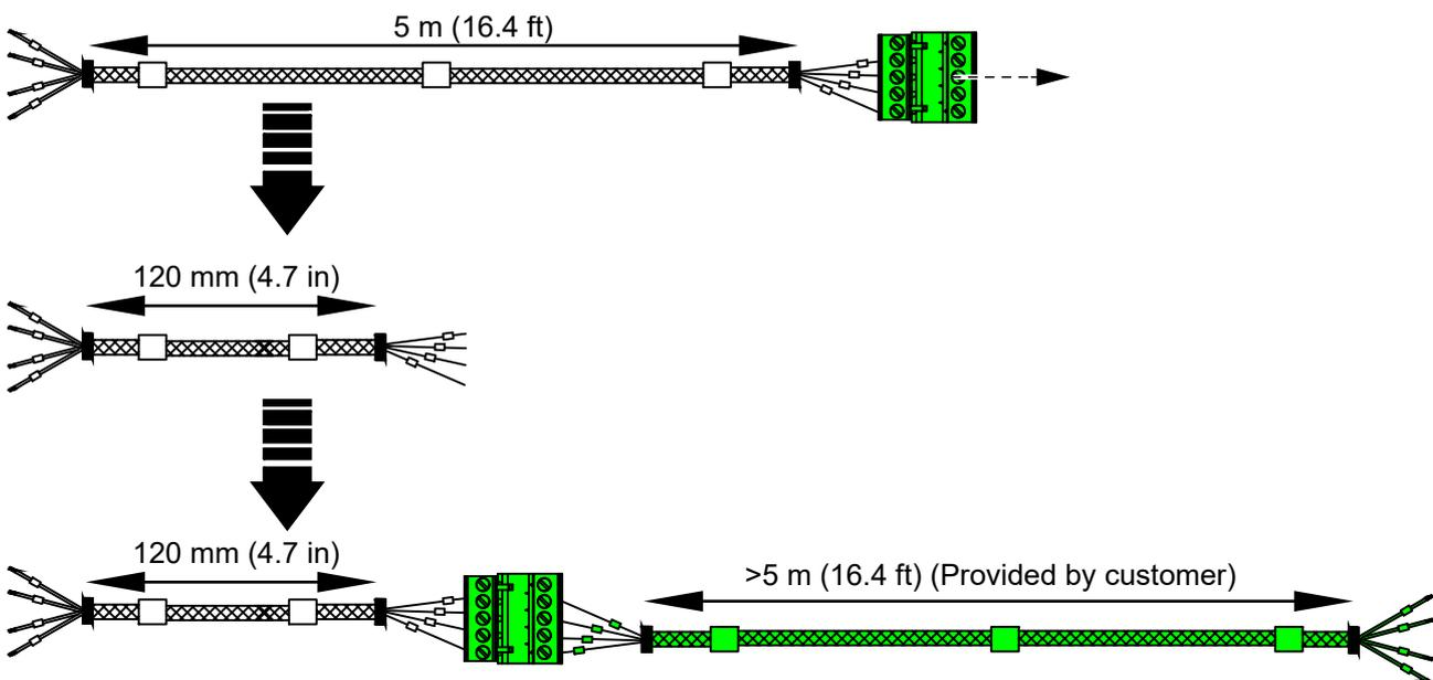
2. Select the extension signal cables according to the *Signal cable specifications*.
