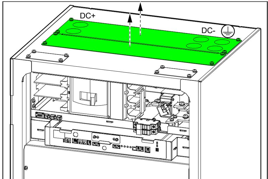
2. Drill or punch holes for cables/conduits in the rear gland plate according to the label on the gland plate.
