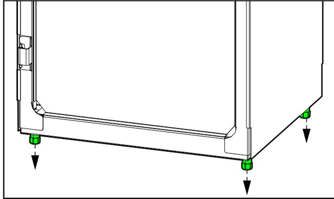
4. Push the second right-most battery cabinet into position, align with the seismic anchoring (if any), and level the battery cabinet as described in step 2 and step 3.
