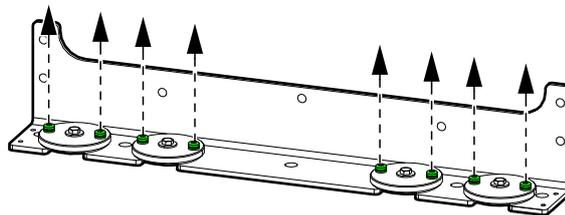
4. Remove the rear seismic bracket.
