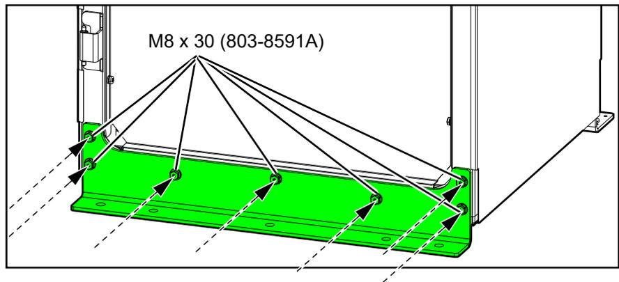
2. Anchor the front seismic bracket to the floor using appropriate hardware for the floor type – the hole diameter in the front seismic bracket is  $\varnothing 14$  mm. The minimum requirement is M12 strength grade 8.8 hardware.
