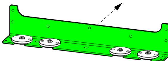
5. Install the rear seismic bracket on the battery cabinet(s).
