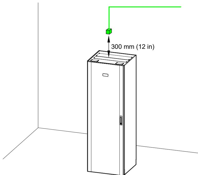
**NOTE:** The temperature sensor measures the ambient temperature. Do not place the temperature sensor close to external heating or cooling equipment which may give an incorrect measurement of the ambient temperature.
