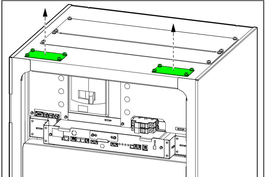
2. Drill or punch holes for cables/conduits and install conduits (if applicable).
