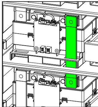
4. Disconnect and remove all signal cables from the battery cabinet. See *Route the Signal Cables to the Switchgear, Rack BMS, and System BMS Ports*, page 31 for details.
