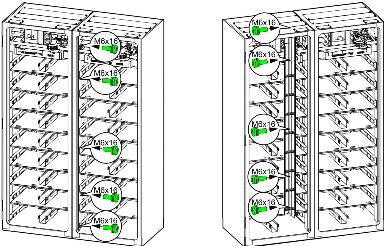
6. Push the third battery cabinet into position, align with the seismic anchoring (if any), level the battery cabinet, and interconnect with the other battery cabinets as described in step 2, step 3, and step 5. Continue until all the battery cabinets are in place, levelled, and interconnected.
