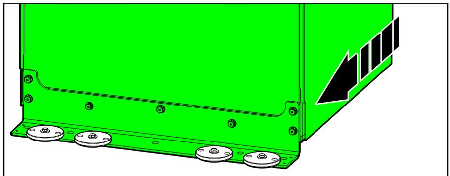
3. Lower the levelling feet until they connect with the floor - use a bubble-leveler to ensure that the cabinet is level.
