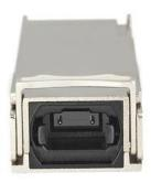
The QSFP-40G-XSR4-AR-ST is an Arista QSFP-40G-XSR4 compatible fiber transceiver module that has been designed, programmed and tested to work with Arista brand switches and routers. It delivers dependable 40 GbE connectivity over fiber cable, for 40GBase-SR4 compliant networks, with a maximum distance of up to 400 m (1312 ft.).
