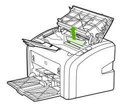
3. When you have removed the jammed media, replace the print cartridge, and close the print cartridge door.
