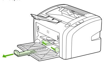
2. Place the envelopes with the side to be printed facing up and the top edge along the left media guide. Stack up to 15 envelopes.
