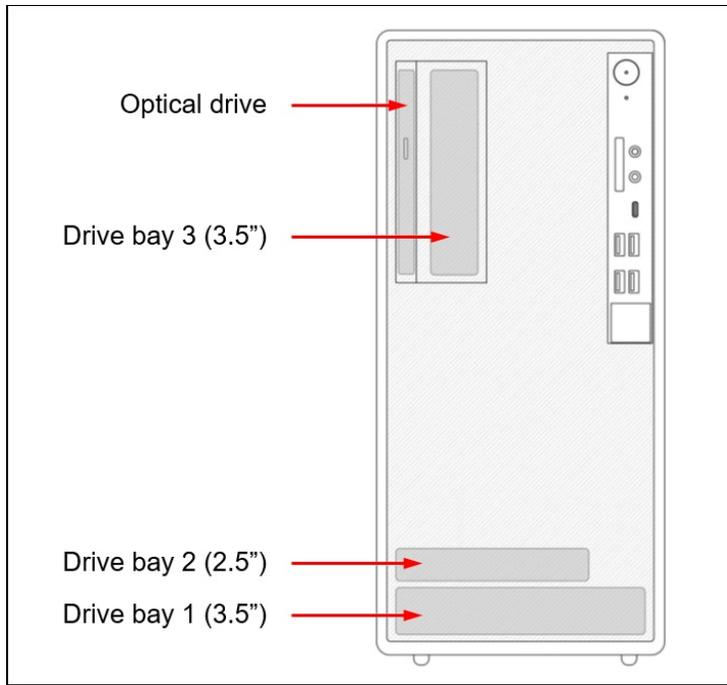
Figure 6. ST50 V2 drive bays (front view)
