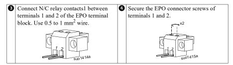
**NOTE:** If the N/C contact is open, the UPS will turn off. Power to the connected equipment will be immediately turned off.
