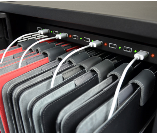
Charge progress LED indicator
