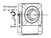
Figure 2-5 Adjust the Angle
