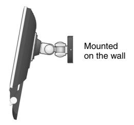
5 Attach the LCD display to the wall, following the instructions in the wall-mounting kit.
