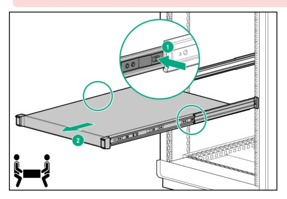
8. Slide the server completely out of the rack.
