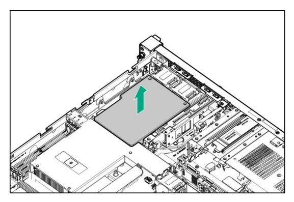
9. Remove the processor air baffle.
