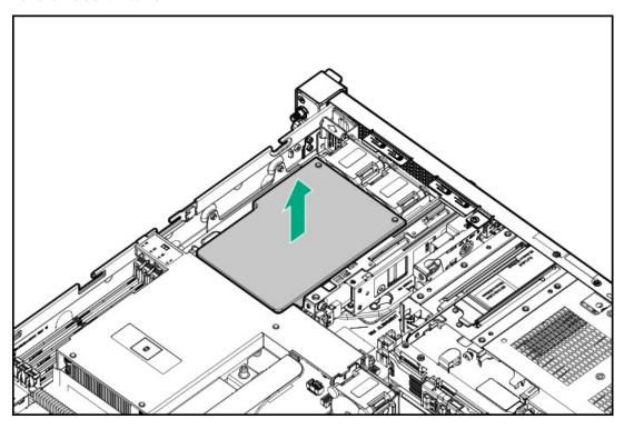
8. Remove the processor air baffle.
