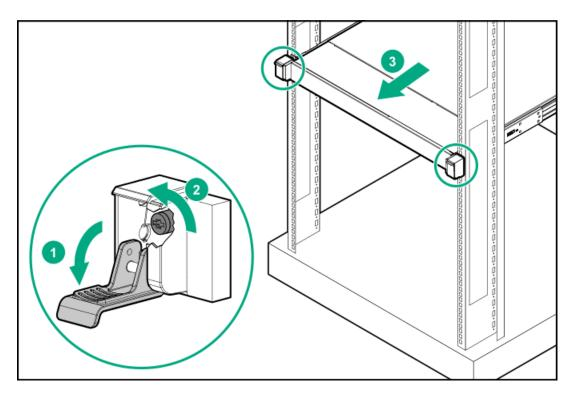
7. Press and hold the rear-end rail-release latches, and then slide the server out of the rack until it is fully extended.
