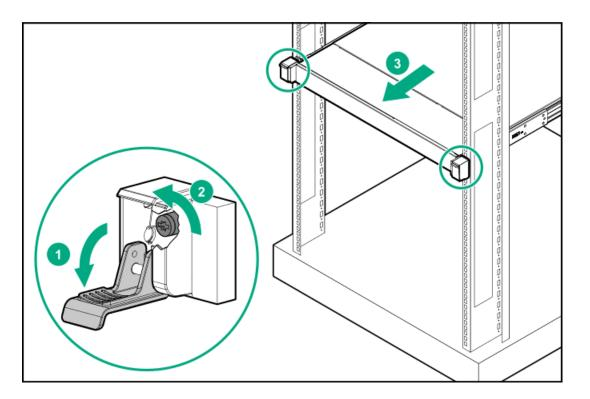
2. Press and hold the rear-end rail-release latches, and then slide the server out of the rack until it is fully extended.
