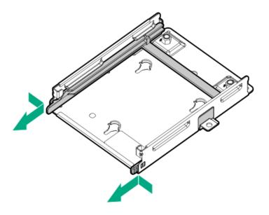
11. Install the type-o controller on the OCP cage rail.
