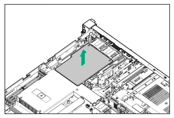
8. Remove the processor air baffle.
