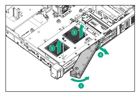
11. Remove the optical drive blank.
