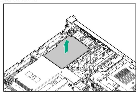
b. Remove the processor air baffle.
