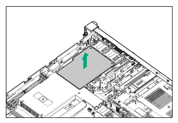
8. Remove the processor air baffle.
