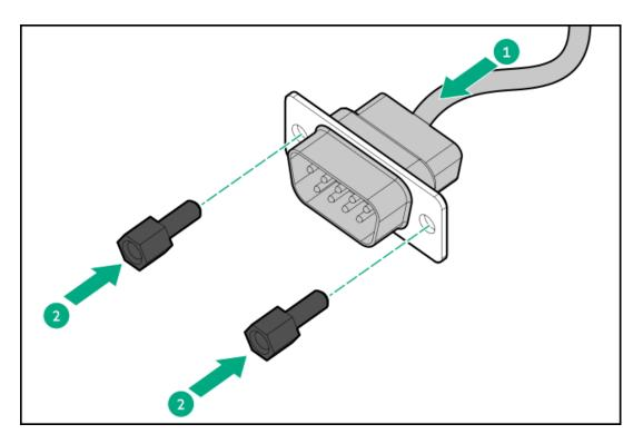
14. Connect the serial port cable to the iLO-M.2-serial module.
