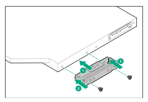
13. Install the optical drive in the optical drive cage.
