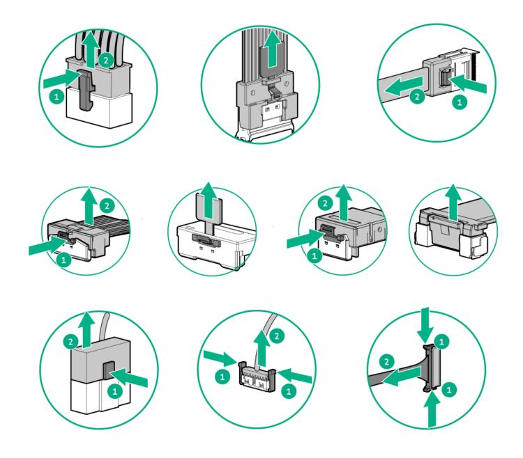
• Remove cables that are no longer being used. Retaining them inside the server can restrict airflow. If you intend to use the removed cables later, label and store them for future use.
