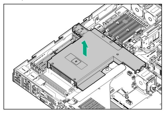
12. Remove the boot device bracket from the server.
