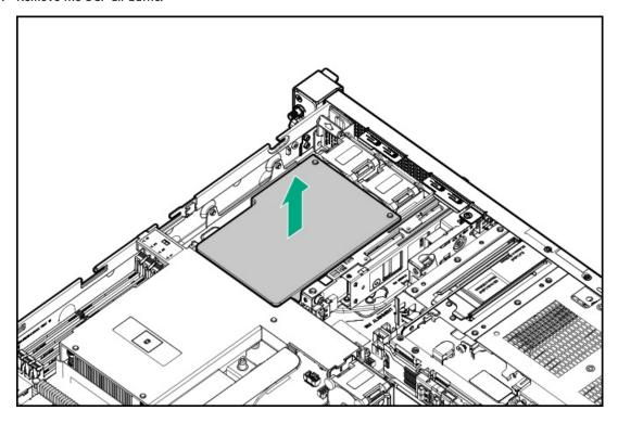
8. Remove the processor air baffle.
