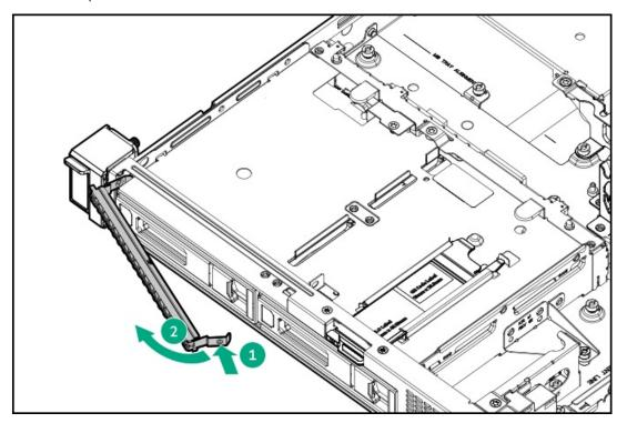
10. Install the optical drive bracket.
