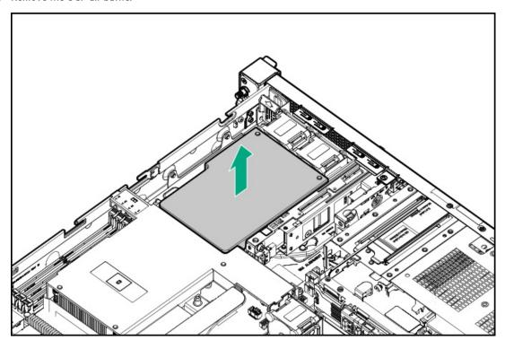
11. Remove the processor air baffle.
