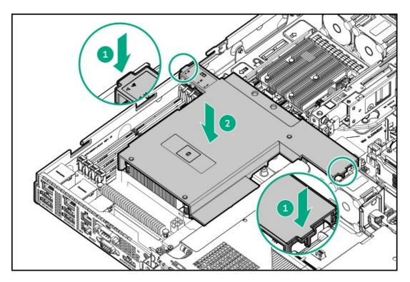
b. Install the OCP air baffle.
