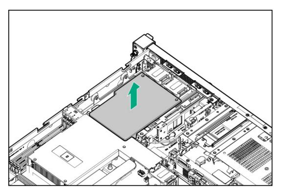
8. Remove the processor air baffle.
