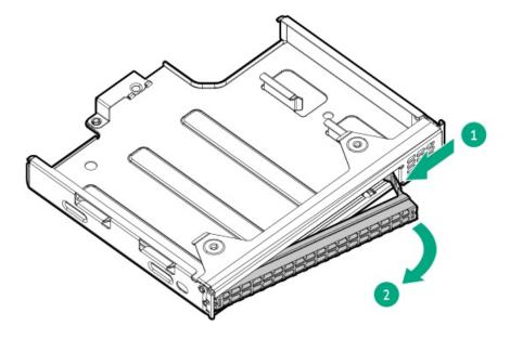
12. Install the optical drive bracket.
