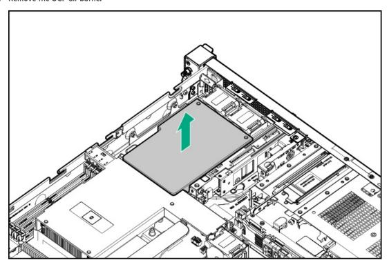
9. Remove the processor air baffle.
