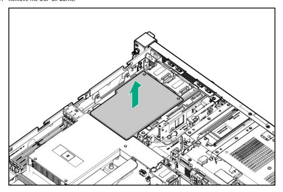
8. Remove the processor air baffle.
