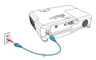
Press the opower button on the projector or remote control. The projector beeps, the Status light flashes blue, and then stays on.
