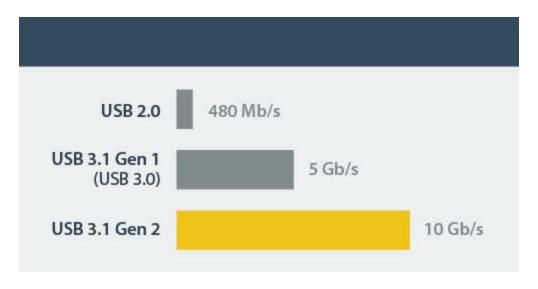
USB 3.1 Gen 2 gives you greater bandwidth and speed with file transfer rates of up to 10 Gbps – twice the speed of USB 3.0 (USB 3.1 Gen 1) technology. It lets you leverage the high performance of the latest SSDs and hard drives, while alleviating bottlenecks in your data transfers.
