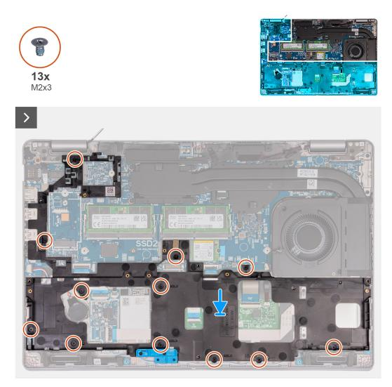
Figure 43. Installing the assembly-inner frame
