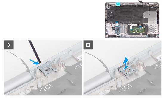
Figure 100. Removing the dummy SIM-card slot filler
