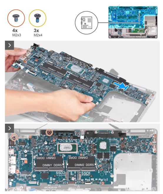
Figure 62. Installing the system board
