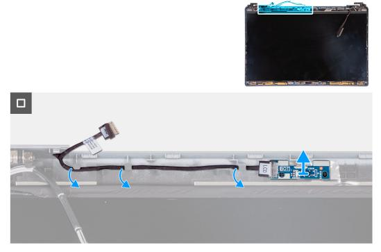
Figure 96. Removing the sensor board
