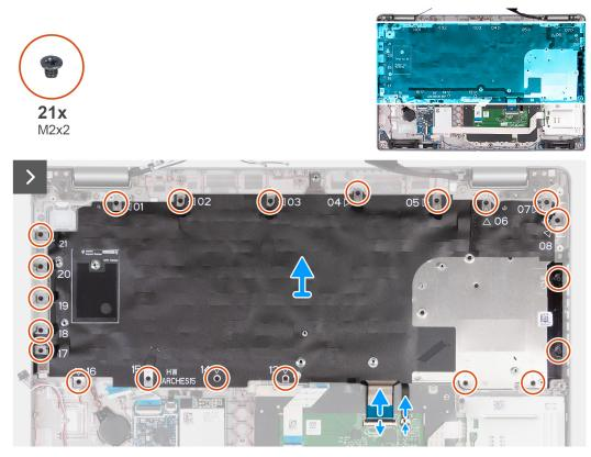
Figure 69. Removing the keyboard
