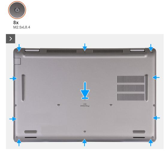
Figure 17. Installing the base cover
