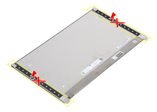
Figure 83. Do not pull and release the Stretch Release (SR) tapes
