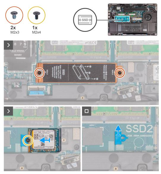
Figure 31. Removing the M.2 2230 SSD from slot 2
