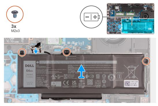
Figure 37. Removing the battery - 64 Wh
