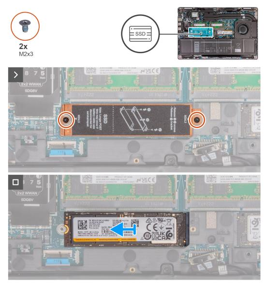
Figure 33. Removing the M.2 2280 SSD from slot 2
