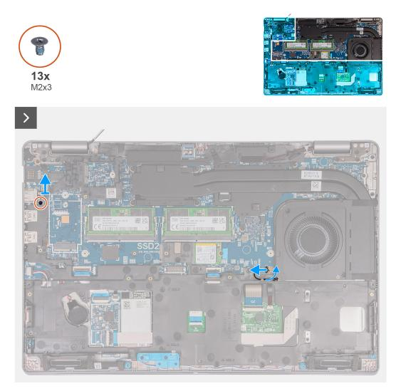
Figure 41. Removing the assembly-inner frame
