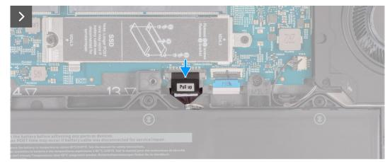
Figure 16. Connecting the battery cable
