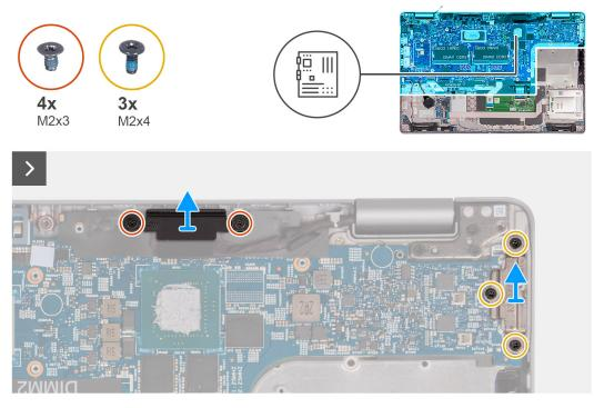
Figure 57. Removing the system board
