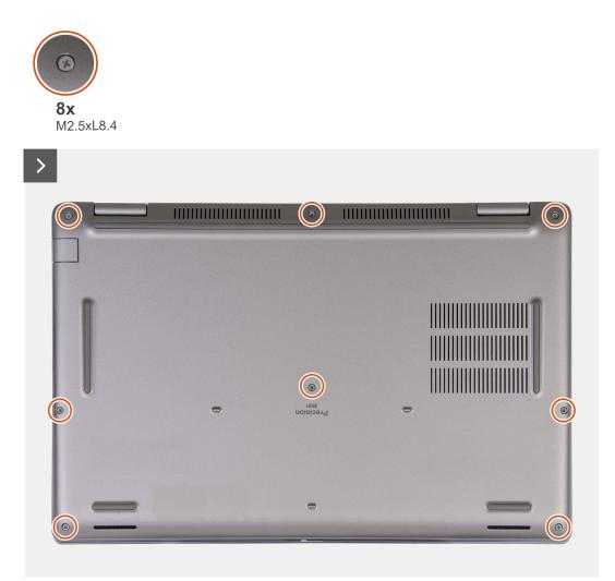
Figure 13. Loosen the captive screws
