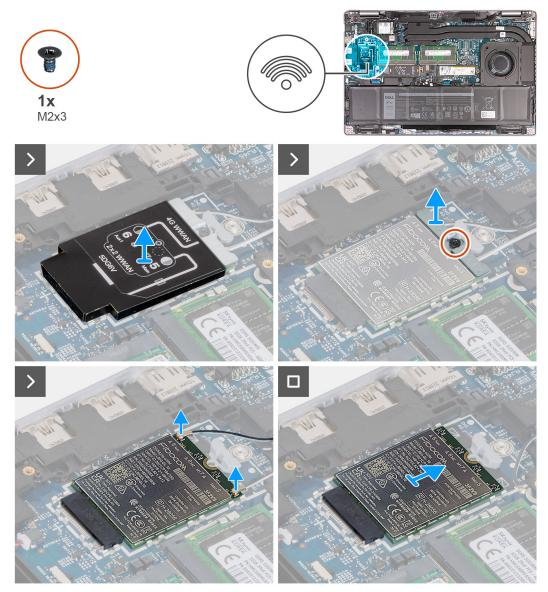
Figure 21. Removing the 4G WWAN card
