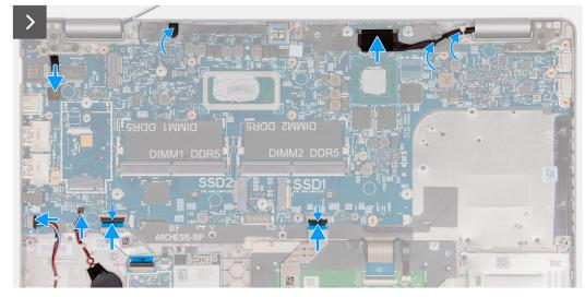
Figure 63. Installing the system board
