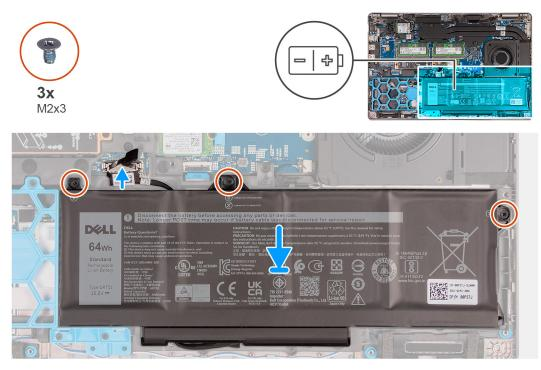
Figure 39. Installing the 64 Wh battery
