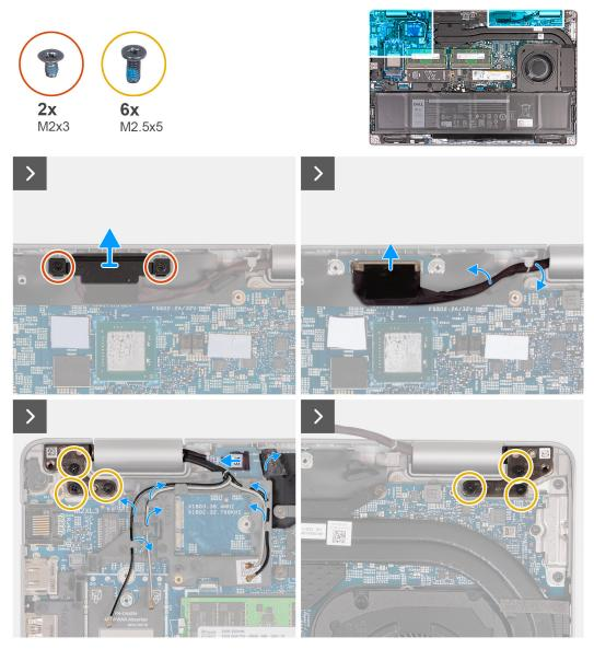
Figure 73. Removing the display assembly
