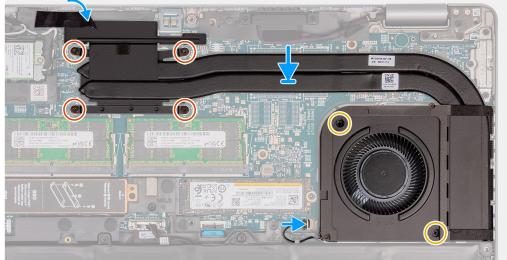
Figure 55. Installing the fan and heat-sink assembly (Integrated GPU)
