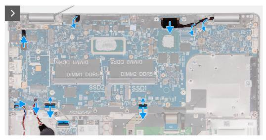
Figure 58. Removing the system board
