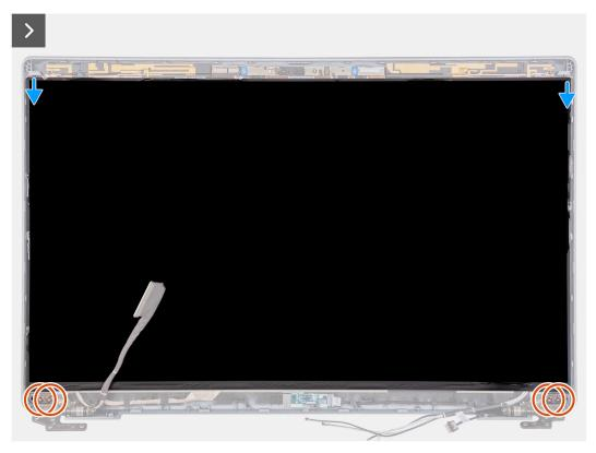
Figure 80. Removing the display panel
