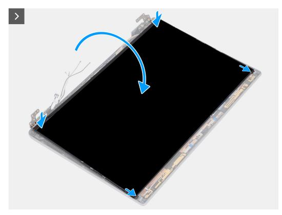
Figure 86. Installing the display panel
