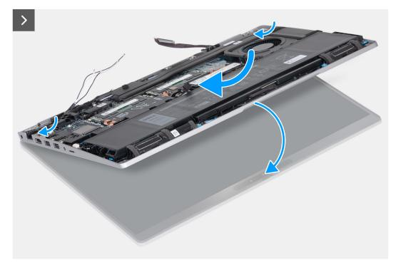
Figure 76. Installing the display assembly
