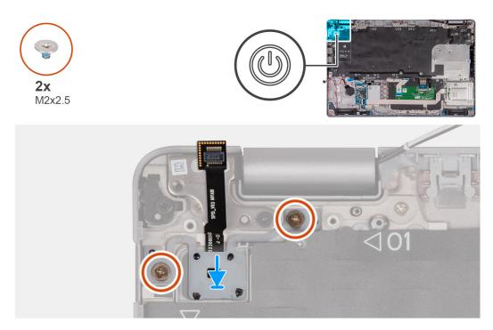
Figure 68. Installing the power button with an optional fingerprint reader
