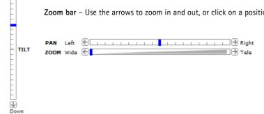
The PTZ controls can be disabled under PTZ > Advanced > Controls, see Controls, on page 27.
