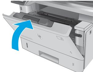
6. Align the toner cartridge with the tracks inside the printer, and install the toner cartridge until it is firmly seated.
