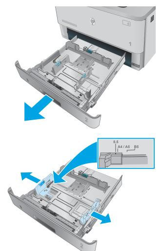
Adjust the paper-width guides by squeezing the adjustment latch on the left guide and sliding the guides to the size of the paper being used.
