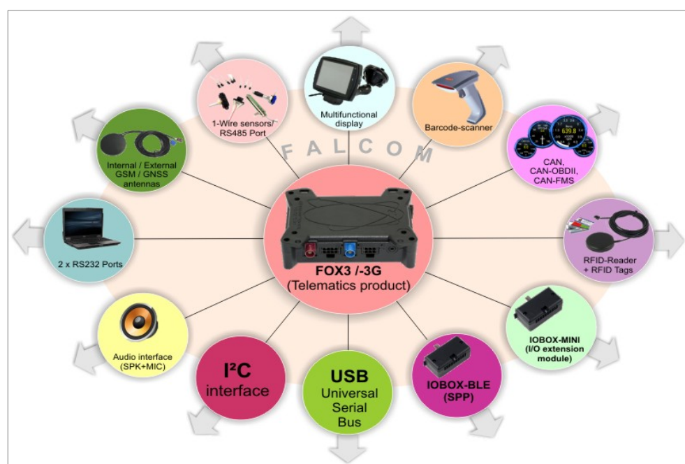
Figure 1: FOX3-2G/3G/4G networking and interfaces to peripheral devices.
