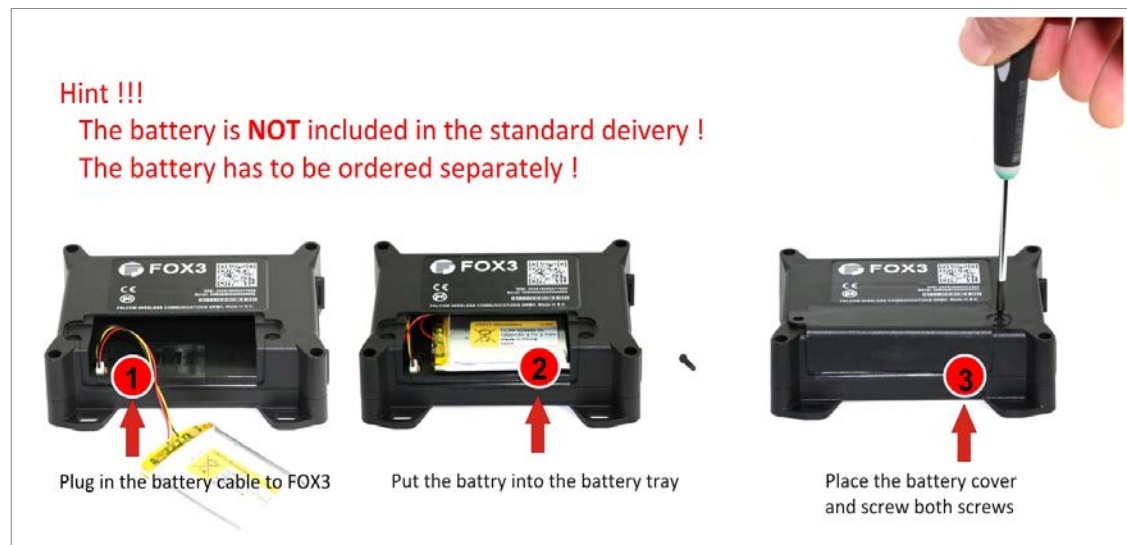
Figure 14.1: Connecting the battery to the FOX3-2G/3G/4G devices
