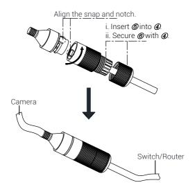
Figure 2-18 Water-proof Accessory Installation
