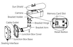
Figure 1-2 Type I Camera Components Overview
