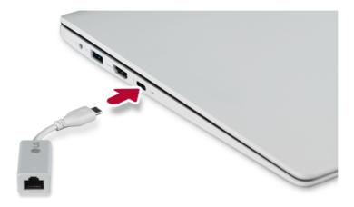
2 Connect the wired LAN cable to the LAN port.
