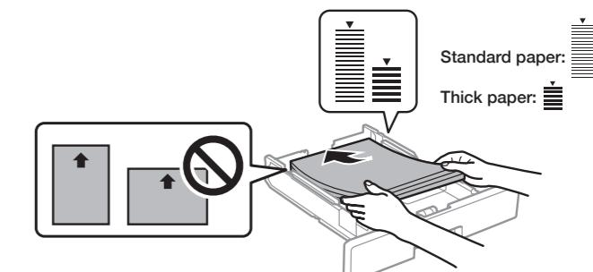
**Note:** Make sure the paper is under the arrow mark for your paper type and loaded against the front edge of the cassette.
