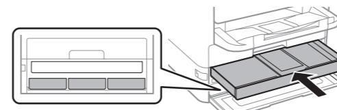
**Note:** The ink packs are keyed to fit into the correct color slots. If you cannot insert the ink tray all the way, do not force it. Make sure the ink pack color matches the color slot on the printer.
