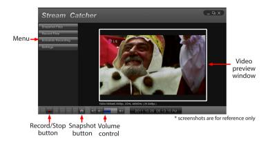
3. Use the Recording controls at the bottom of the window, as necessary.
