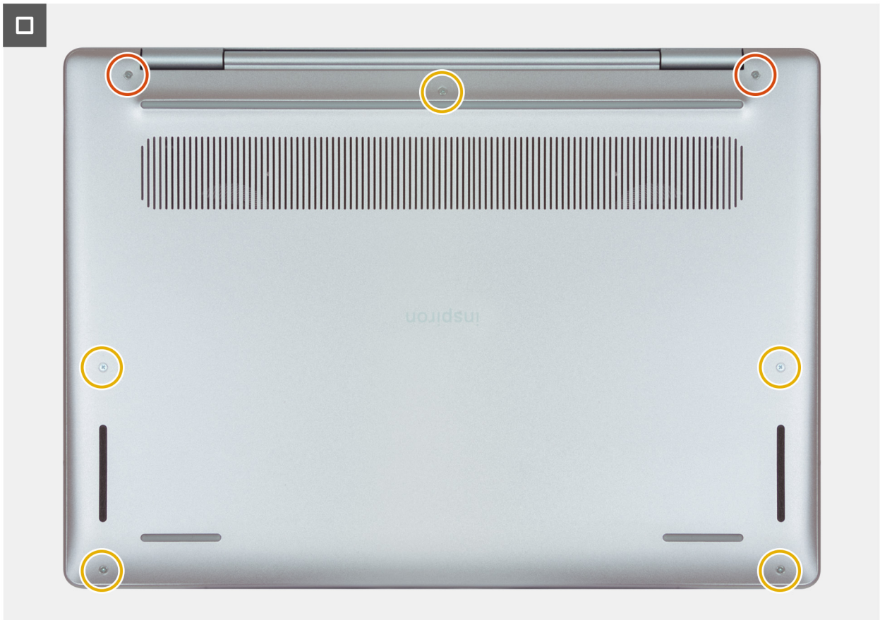
Figure 15. Installing the screws
