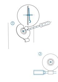
2. Attach the magnetic base to the metallic plate. Attach the Outdoor Cam Pro / Outdoor Cam onto the magnetic base.
