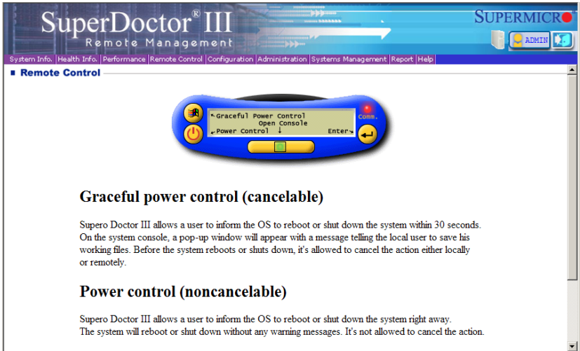
Figure 5-7. SuperDoctor III Interface Display Screen (Remote Control)
