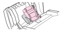
7. Make sure that both sides of the assembly are secured by the green hooks.
