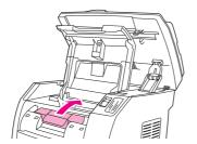
4. Lift the imaging drum straight up to remove it from the device.
