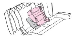
8. Make sure that both sides of the assembly are secured by the green hooks.
