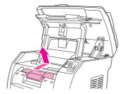
4. With both hands, grasp the side of the media that is most visible (this includes the middle), and carefully pull it free from the device.
