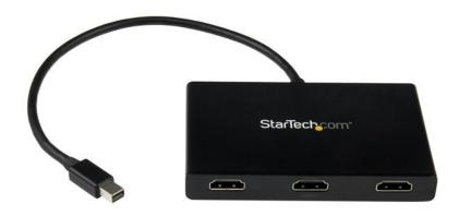
This MST hub lets you connect three HDMI monitors to your Mini DisplayPort computer. MST works on any Windows® device that supports DisplayPort 1.2, such as models of the Lenovo™ Think Pad® and Microsoft® Surface™. When connected to earlier revisions of DisplayPort, such as DP 1.1 the MST hub acts as a video splitter.
