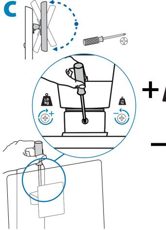
Increase Lift Strength If the mounted weight is too heavy or this product does not stay up when raised, then you'll need to increase Lift Strength:
