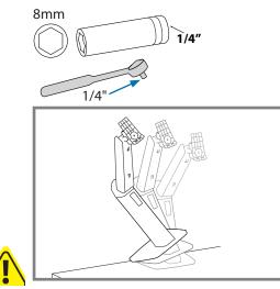
CAUTION! Tipping Hazard. Support the stand until the clamp is securely tightened. Failure to follow these instructions may result in the stand tipping over causing possible equipment damages and or personal injury.
